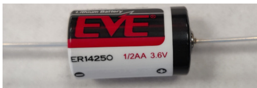
Battery ER14250 soldered (P/N 13053566)
