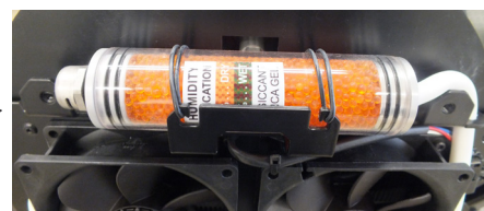
Silica gel desiccant in tube in the fixture head
