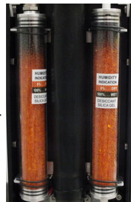
Silica gel desiccants in the fixture arm
