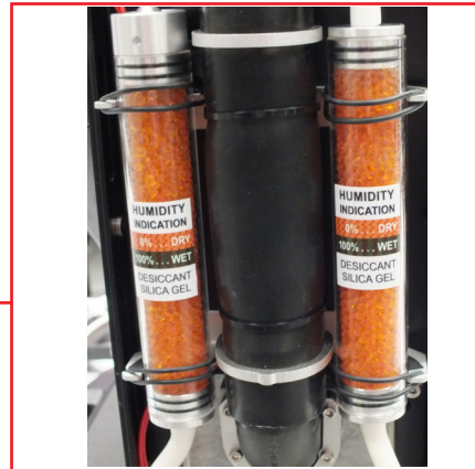
Silica gel desiccants in the fixture arm
