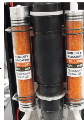
Silica gel desiccants in the fixture arm
