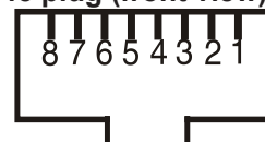
RJ-45 plug (front view):
