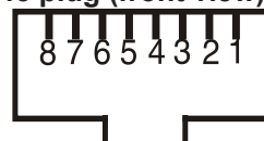
RJ-45 plug (front view):
