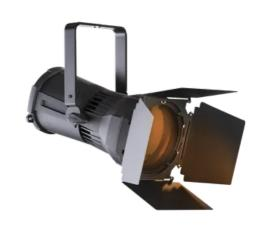
The RGBA LED colour combination provides a high CRI and allows designers to produce warm, rich, amber tones that are normally difficult to achieve. Other features include smooth CMY & RGBA colour control, 18-bit dimming and Tungsten emulation, with both selectable & variable colour temperatures providing total output control.
