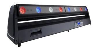
An array of individually controlled 15W RGBW LED modules equally spaced along the strip with fully adjustable zoom from 8-67 degrees. The strip itself has a very fast 270 degree tilt movement which can be precision indexed or programmed to produce rapid sweeping movements. Pre-programmed colour macros and pixel control makes this fixture quick and easy to programme. Tungsten lamp emulation and fade effects at 2700 K and 3200 K are included. Wireless technology CRMX is available as an option.
