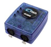
Cyber Pro II is using a new USB-DMX interface with 3 DMX universes + 4 ArtNet universes (via the computer network interface) and miniSD CARD memory. Cyber Pro II is the only interface which is compatible with new Cyber Control II + Easy Stand Alone PRO software and therefore offers multiple extra functions. Cyber Pro II interface come with a powerful standalone features: miniSD card memory, multi-zone, sunset/sunrise and daylight saving function, IR receiver and more.
